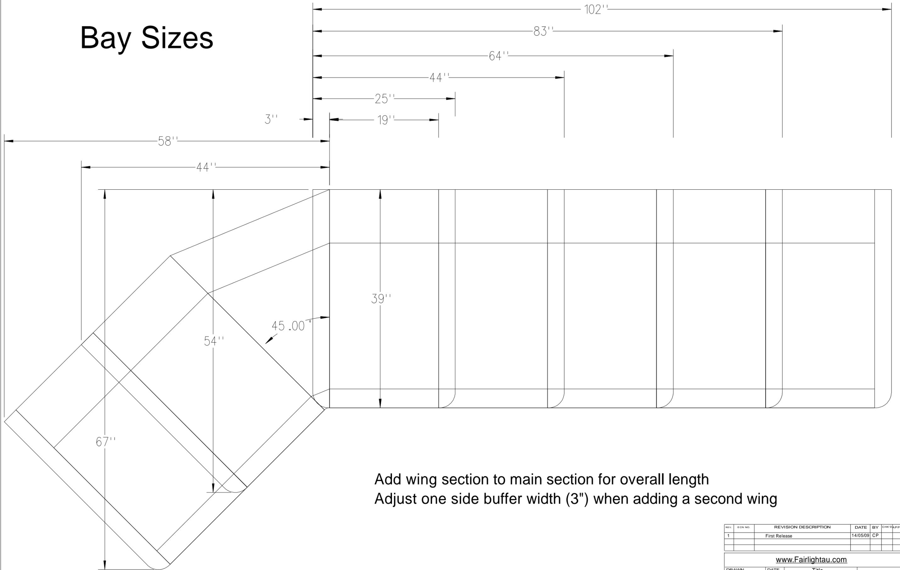
Add wing section to main section for overall length
